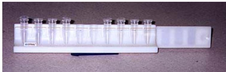
Fig. 2.3 Dynal particle concentrator: Microcentrifuge tube holder containing tubes, with magnet bar half way in place.
