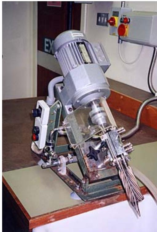
Fig. 1.1 (a) Mechanical potato peeler (Imperial Machine (Peelers) Company Ltd).
