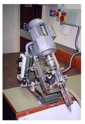
Fig. 1.1 (a) Mechanical potato peeler (Imperial Machine (Peelers) Company Ltd). (b) Pollähne press (Meku).
