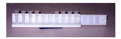
Fig. 2.3 Dynal particle concentrator: Microcentrifuge tube holder containing tubes, with magnet bar half way in place.
