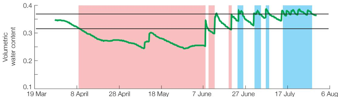
**Figure 1** Variation in the volumetric water content of soil over time at SCRI showing periods when roots were likely to be limited by mechanical impedance (pink) and shortage of oxygen (blue).
