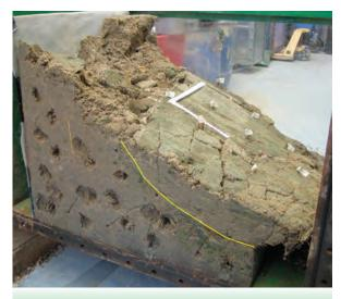
Figure 1 Model of rooted slope following testing in the centrifuge at 15 x gravity. Yellow line indicates failure plane.
