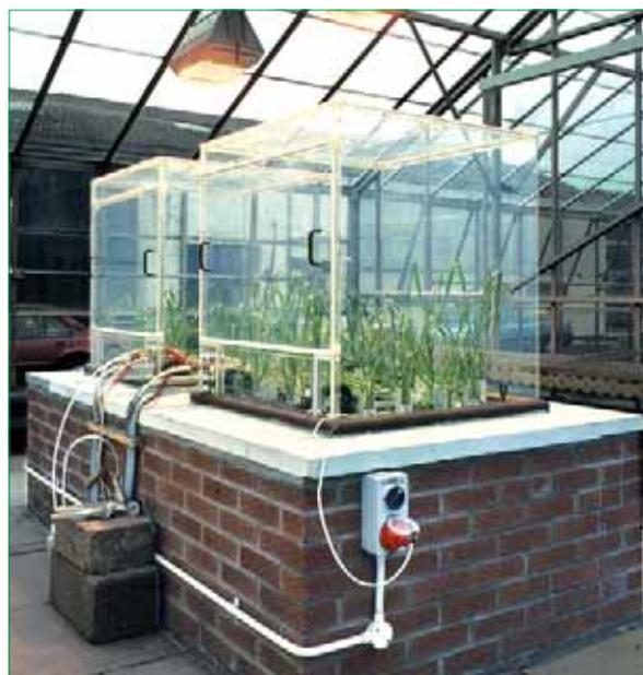
Controlled growth chamber with elevated CO<sub>2</sub>.
