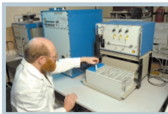
Stable Isotope Facilities. Gas samples being prepared for automated analysis of ^{13}\text{C} and ^{18}\text{O} in \text{CO}_2 .
