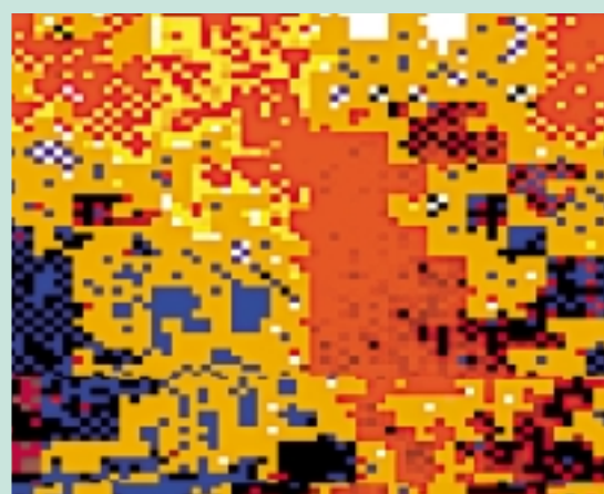
Figure 3 Simulation of chemically-reactive solute flow in a fractal soil structure (brown). Red to blue denotes high to low concentration respectively.
