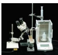
2) Ethanol Sorptivity – removes impact of repellency, related to pore structure.
