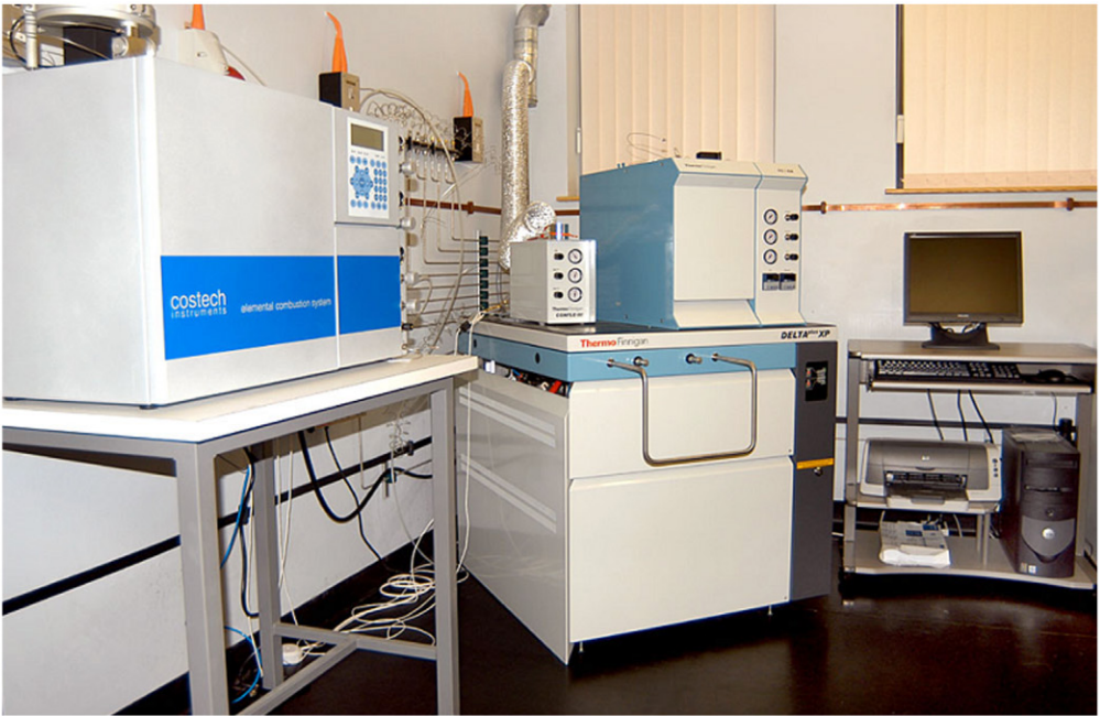
Figure 1. FEL IRMS instrumentation. Thermo Finnigan De DeltaPlus XP with a Costech Elemental Combustion System, Thermo Finnigan TC/EA and a Thermo Finnigan ConFlo III Interface Unit
