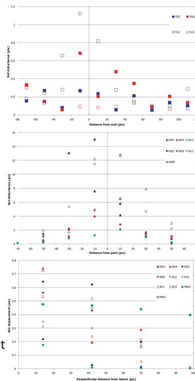
Figure 4. Soil disturbance around taproots, joints and lateral roots in herringbone and dichotomous root patterns
