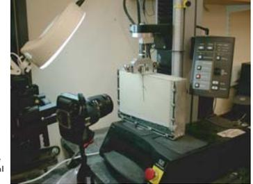
Figure 1. Experimental setup. Roots were pulled out at a constant rate while digital photos were taken at regular intervals.
