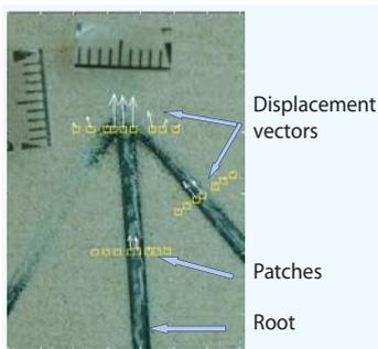
Figure 3. Soil patches (20 pixels) and displacement vectors
