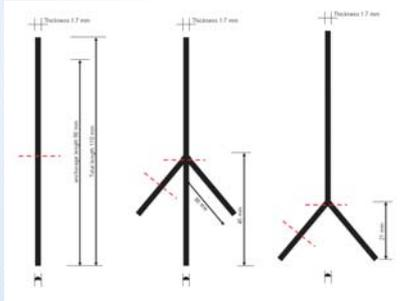
Figure 2. Idealised root architectures used in this study. Red dashed lines show the planes where soil movement was traced.
